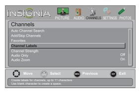
3 Press ▲ or ▼ to highlight Channel Labels, then press OK. The Channels-Channel Labels screen opens with the channel number field highlighted.
